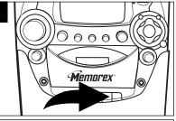
When the tape reaches the end, the auto-stop mechanism activates, the PLAY  $(\blacktriangleright)$  and RECORD (●) buttons are released and the tape motor shuts off. Press the STOP/EJECT (■▲) button to open the Cassette Door and remove the tape.
